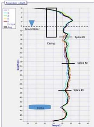
Example of measured temperature for each string vs depth
